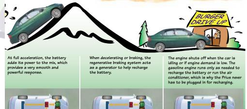
and the generator, can either charge the batteries or power an electric motor that drives the wheels.
