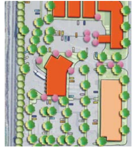
FIGURE 3 A thriving light industrial base of business was in need of room to grow. Infill development provided the answer. Again, reconfiguring surface lots provides room for new tenants and creates a more unified streetscape. In the plan image, dark buildings are new and light orange are existing with adaptive reuse.
