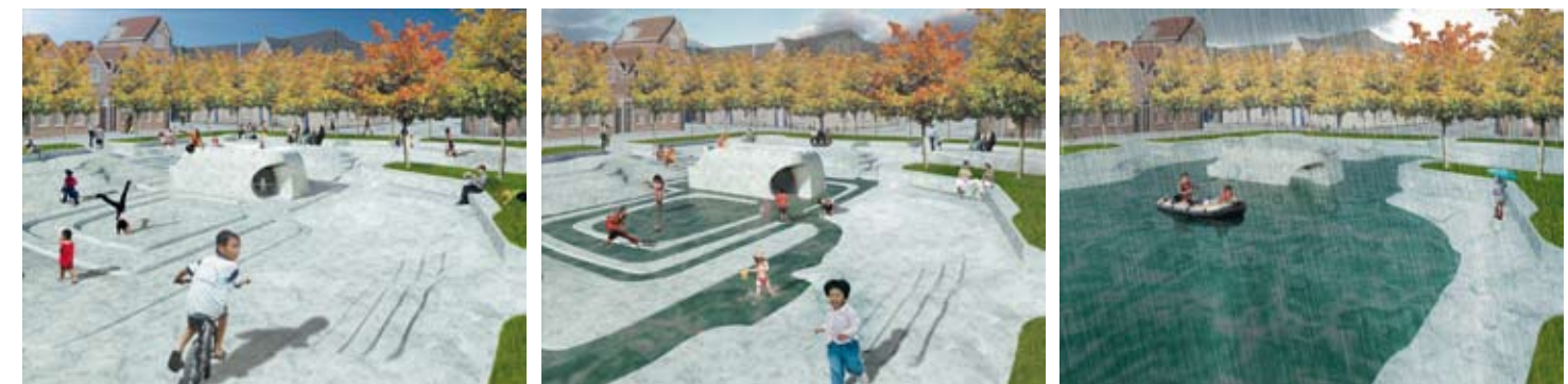
Design Bloemhofplein, depicting different weather situations. Water plazas are an innovative way to deal with heavy rainfall.
