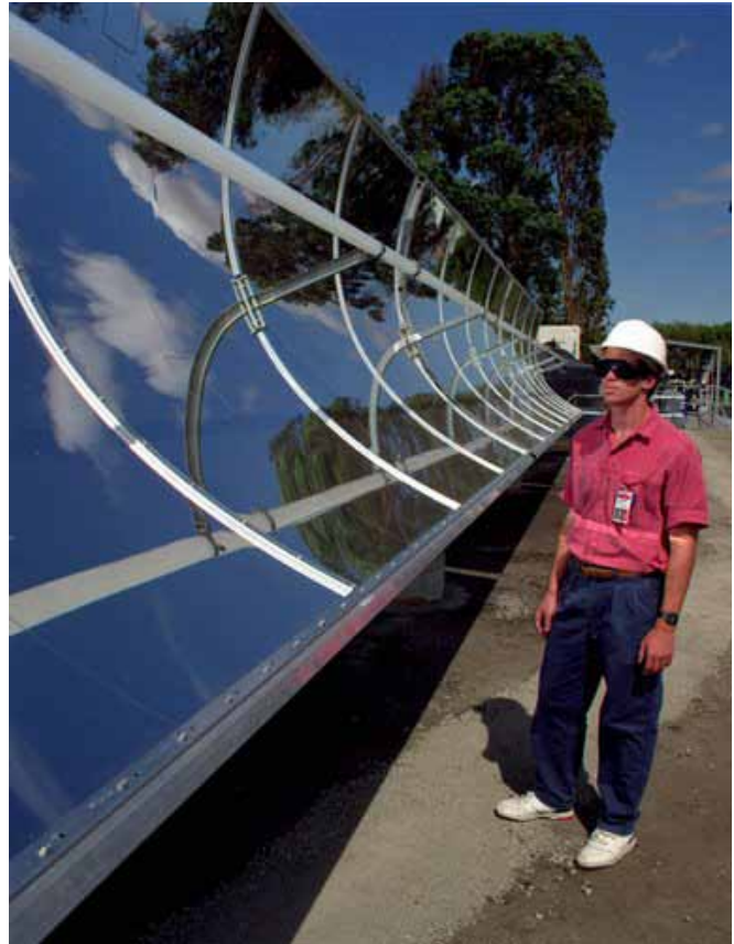
This solar installation on a Superfund site in Livermore, California, used concentrated sunlight to destroy volatile organic compounds in the groundwater. (Image Courtesy Warren Gretz/NREL.)
