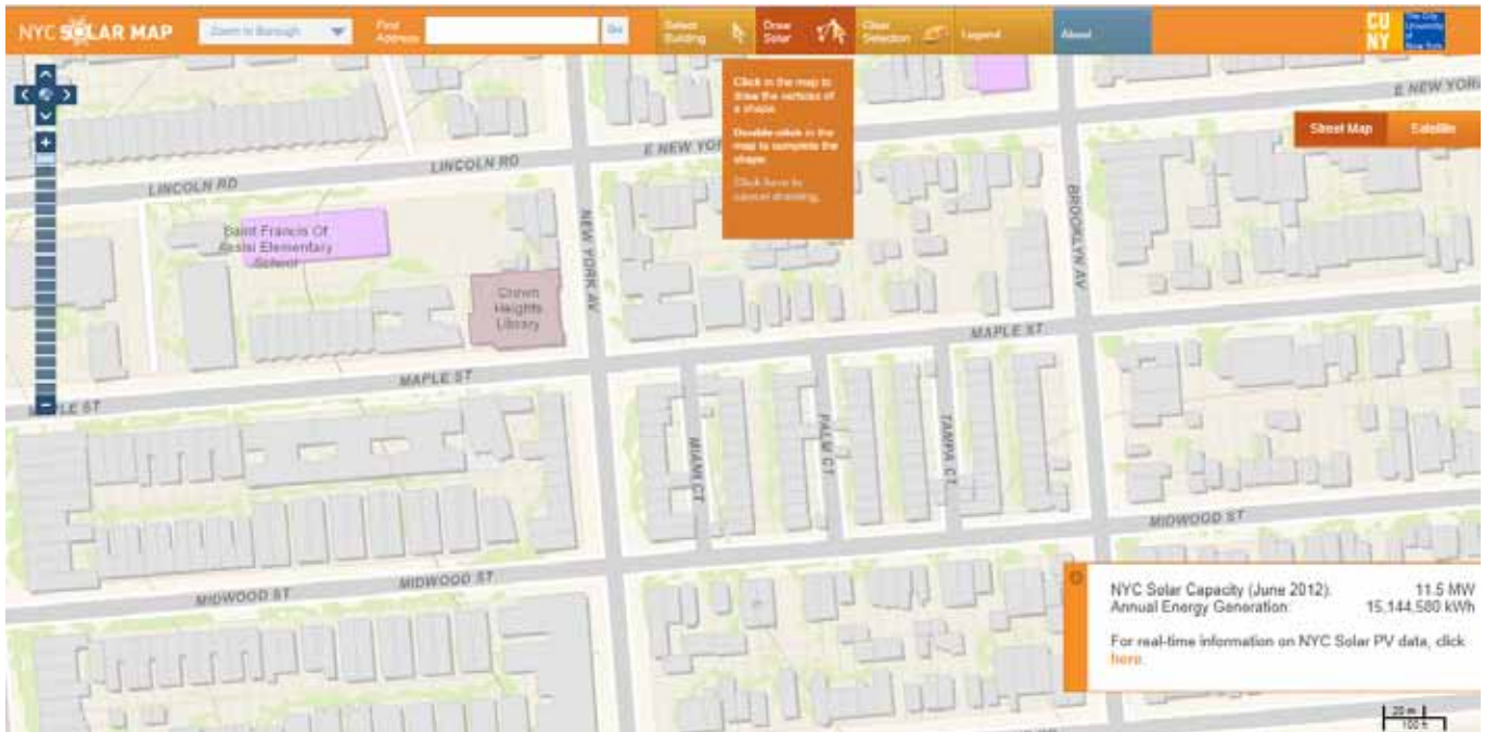
The Draw Solar tool in New York City's solar map allows users to draw a solar installation and immediately generate information on the installation including cost, financial metrics, electricity bill savings, environmental impacts, and available incentives. (Image courtesy of http://nycsolarmap.org/ )
