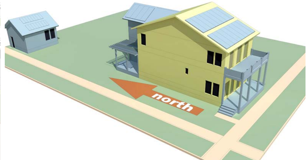
This diagram (above) illustrates how housing design can be optimized for solar heat gain and control as described.
