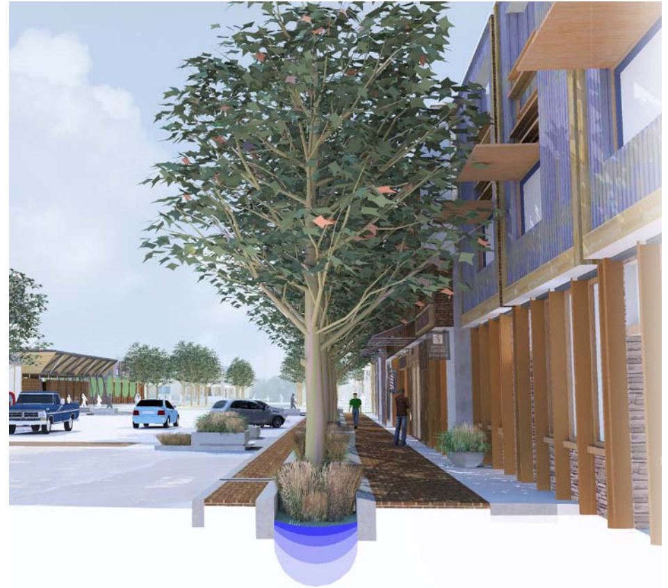
The Downtown Streetscape employs decorative planter zones to capture street and sidewalk stormwater runoff for storage and infiltration. Natural systems-based stormwater features can provide many functional and aesthetic benefits when incorporated into park and open space design.
