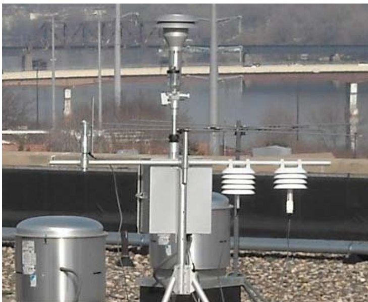
This mobile air quality monitor is a new tool being tested by the City to measure fine particulate air pollution for specific activities.
